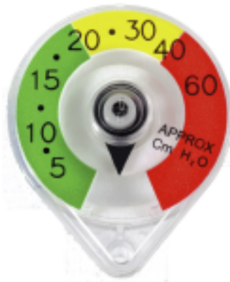
Color-Coded Manometer: green 0 - 20 cm H 2 O, yellow between 20 - 40 cm H 2 O and red over 40 cm H 2 O.
