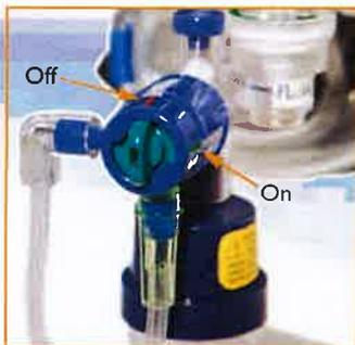
On/Off nebulizer switch incorporated in new integrated design
